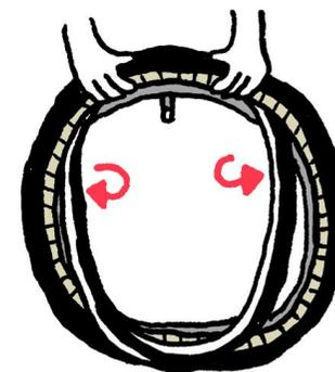
11 - RENTRER LE FLANC DU PNEU DANS LA JANTE, EN PARTANT DE LA VALVE, À MAINS NUES. ÉTIRER LE PNEU VERS SOI SI LE MONTAGE DEVIENT DIFFICILE VERS LA FIN.
